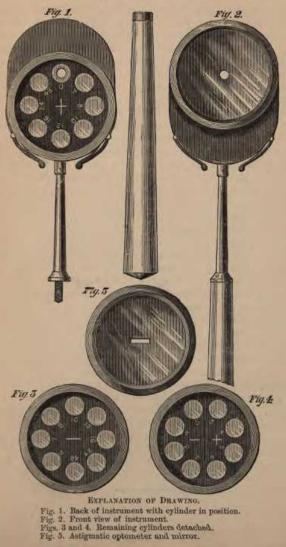
Great care was taken to have the mirror, which is concave, seven inches' focal distance, ground exceedingly thin—as thin almost as a metal mirror—while all the surrounding brass work is so beveled away that as little impediment as possible is offered to the passage of the rays, thus rendering the image perfectly distinct, and I think unusually brilliant.
