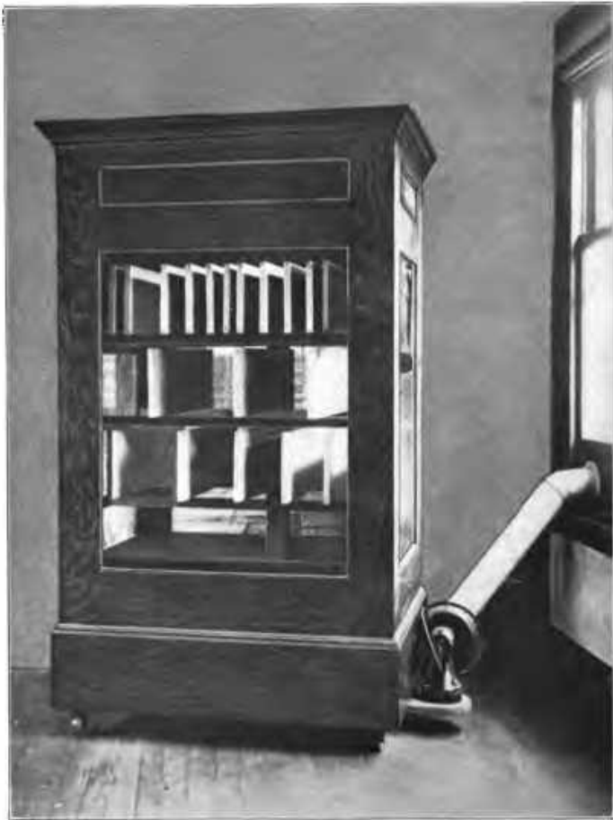
Figure 1 Test Board Drying Cabinet Supplied With Clean Out-of-Door Air.
