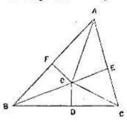
any triangle. Bisect BC in D, and through D draw DO perpendicular to BC. Bisect the angle BAC by AO.
